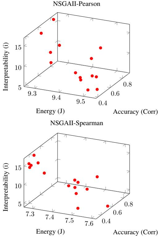
Fig. 6. NSGA-II was used to create a Pareto front of non-dominated points. The Pearson Correlation Coefficient is depicted in the first plot, while the Spearman Rank Correlation is depicted in the second.
