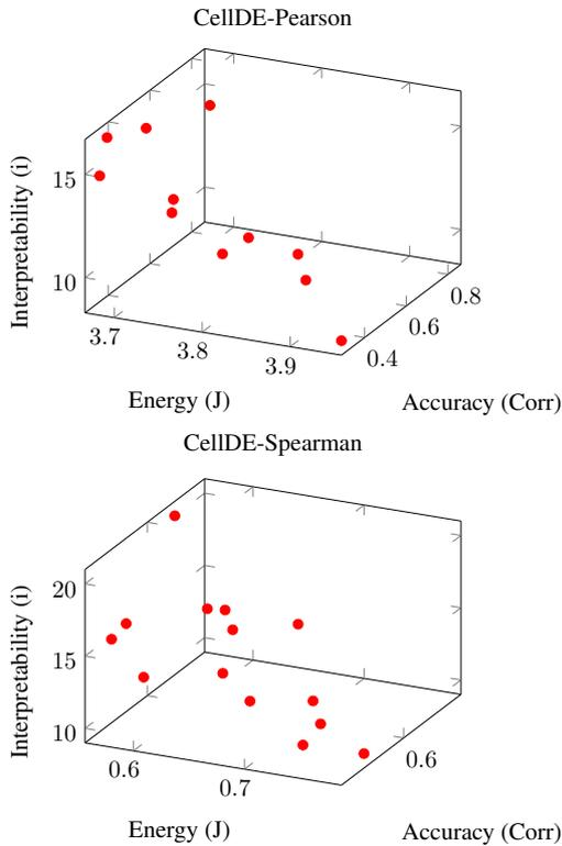
Fig. 2. CellIDE was used to create a Pareto front of non-dominated points. The Pearson Correlation Coefficient is depicted in the first plot, while the Spearman Rank Correlation is depicted in the second.
