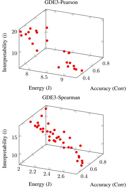
Fig. 4. GDE3 was used to create a Pareto front of non-dominated points. The Pearson Correlation Coefficient is depicted in the first plot, while the Spearman Rank Correlation is depicted in the second.
