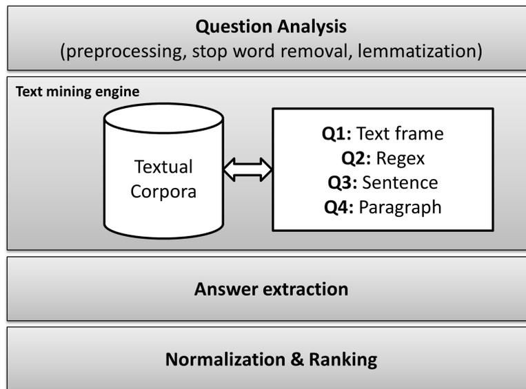
**Fig. 1:** Overall view of a pipeline designed to answer the multiple-choice tests. First of all, questions and answers need to be pre-processed. After this, a text mining engine is in charge of mining reinforced co-occurrence patterns. Then, these patterns are analyzed. Finally, the results are normalized and a ranking of potential choices is delivered
