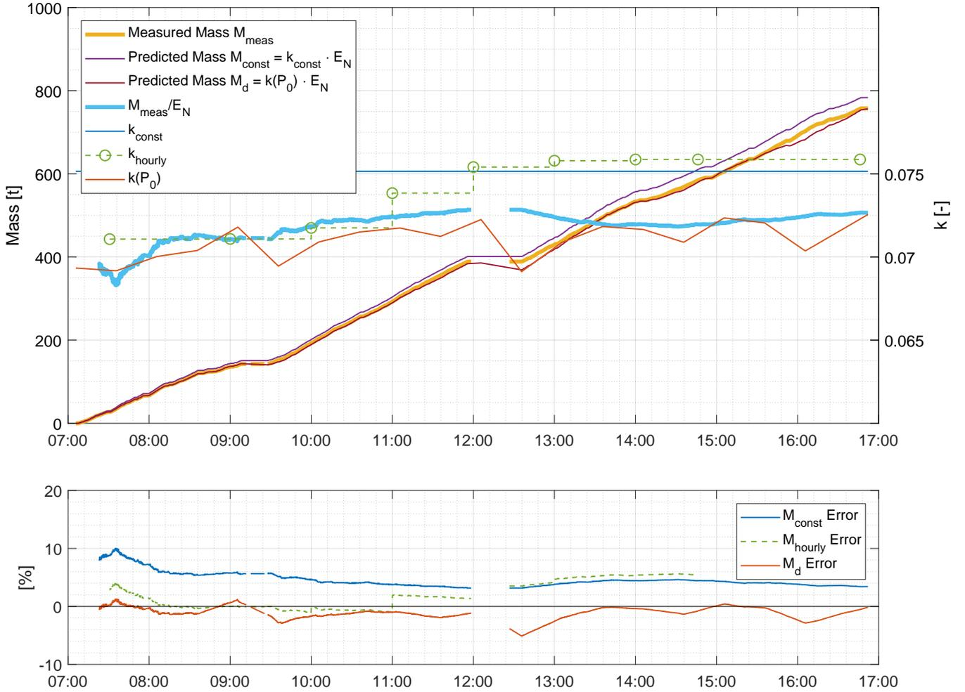
Fig. 4. Validation working period, again comparing  $k_{\text{const}}$ ,  $k_{\text{hourly}}$  and  $k(P_0)$ .
