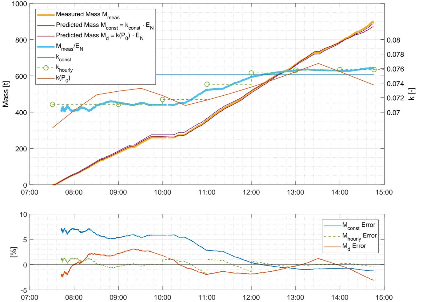
Fig. 3. Working period for training the regression model with comparison of different  $k$  models: constant value  $k_{\text{const}}$ , hourly values  $k_{\text{hourly}}$  and state-dependent model  $k(P_0)$ . The bottom plot depicts the resulting relative error between predicted and measured mass flows.
