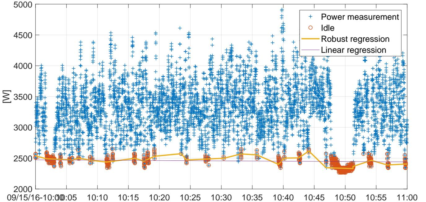
Fig. 2. Example power measurement with idle power estimation via linear regression and robust piecewise regression
