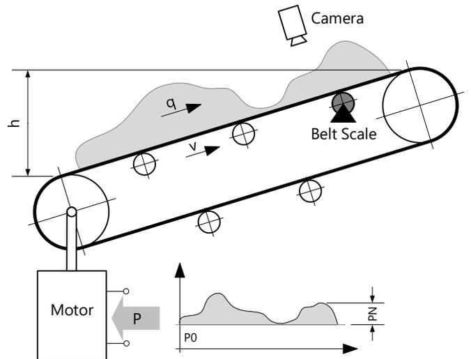
Fig. 1. System under study consisting of conveyor belt with electric drive motor and reference measurement system with Belt Scale and camera system for volume measurement.
