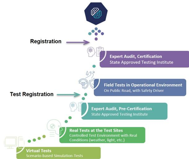
Figure 2: Sketch of the steps required to verify trustworthy AI in the case of autonomous driving.
